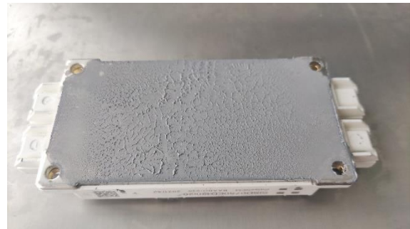
Example of good thermal grease coverage (module removed after mounting)
