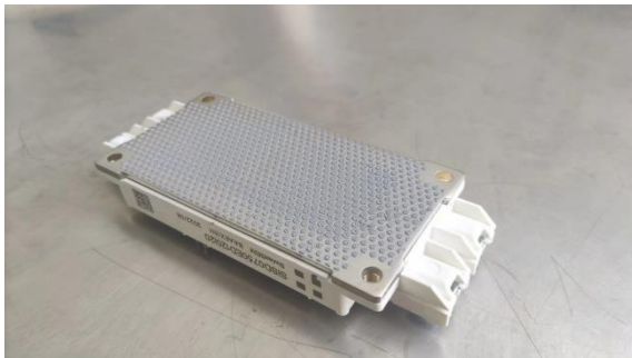
Example of an ED-type module after stencil printing
