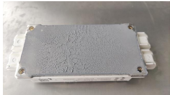
Example of good thermal grease coverage (module removed after mounting) 导热硅脂覆盖良好的示例 (模块安装后拆除)
